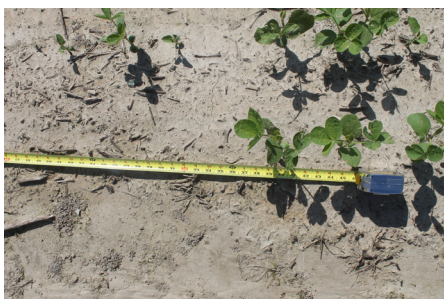
Figure 5. Measurement to demonstrate accuracy of the “skipulator” planting system. In this case, the target was a 40-inch skip and was close.
